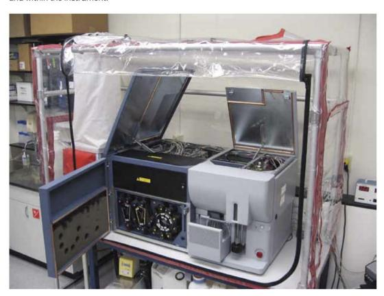
THE "BIOAERSOL IMPACT SAMPLER" SYSTEM CONSISTED OF A FLOW REGULATED VACUUM PUMP AND A AIR CONCENTRATOR SAMPLER CAPSULE.
