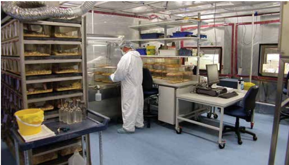
< INTEGRATED ULTRA- CLEAN HOUSING AND PROCEDURAL SPACE WITH TWO BIOSAFETY CABINETS DOCKED TO EXTERIOR OF bioBUBBLE CLEAN ROOM
