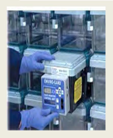
EACH VENTILATED RACK IS CONNECTED TO A DETECTION SYSTEM, MONITORING SET POINT VARIATIONS IN **ENVIRONMENTAL CONDITIONS** (e.g. TEMPERATURE, HUMIDITY, LIGHT INTENSITY AND POWER FAILURE) AND SENDING **IMMEDIATE ALERTS VIA SMS** AND EMAIL MESSAGES TO **SMARTPHONES**
