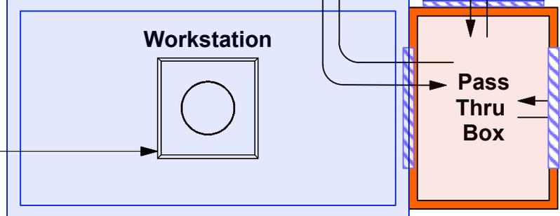
Workstation docks to Pass-Thru Box and to Positive Pressure Cleanroom
