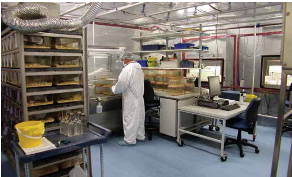
< INTEGRATED ULTRA-CLEAN HOUSING AND PROCEDURAL SPACE WITH TWO BIOSAFETY CABINETS DOCKED TO EXTERIOR OF bioBUBBLE CLEAN ROOM
